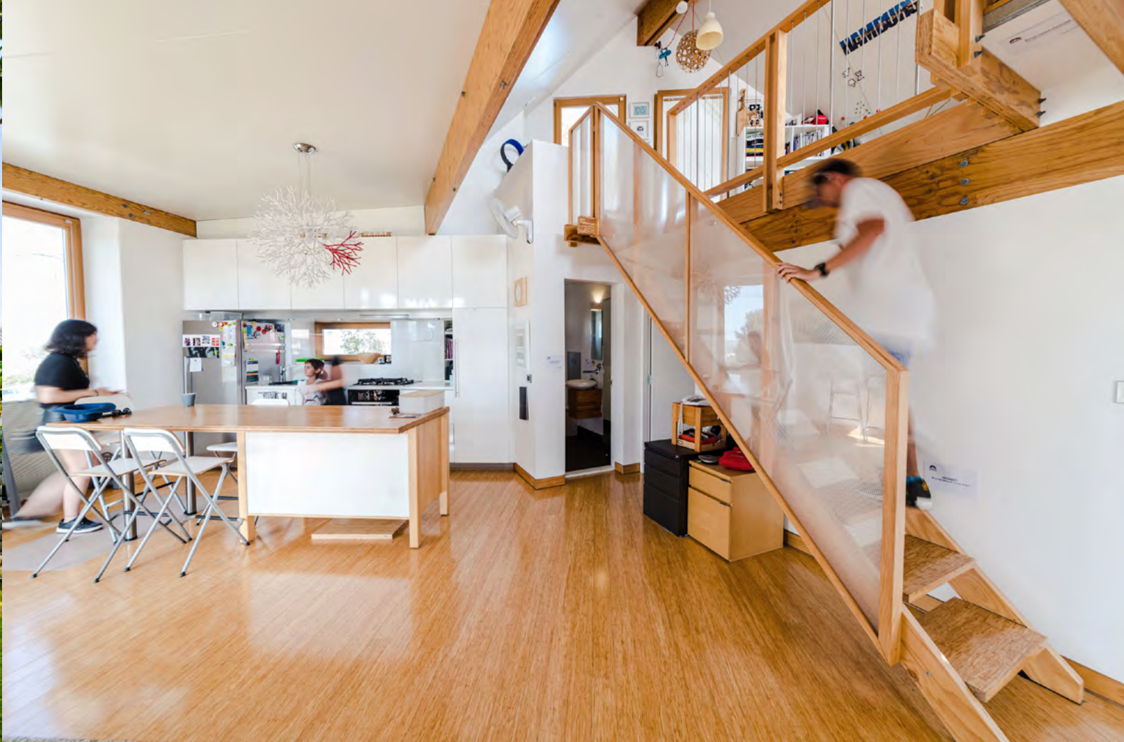
↑ Christian and Deepti live in the upstairs unit with their two children. The strawbale infill walls are finished with lime and sand render and provide excellent thermal and acoustic insulation, important as the house is situated right on a busy road.
